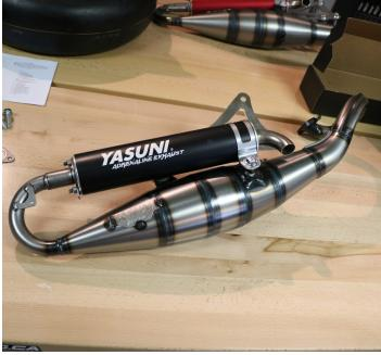
NOTE - The center stand can be retained with the Yasuni R exhaust. This model has a restriction inside the chamber. **It is required to remove the chamber restriction for best performance.**
