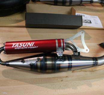
NOTE - The center stand can be retained with the Yasuni Z exhaust. This model has a restriction inside the chamber and the silencer. It is equired to remove the chamber restriction for best performance.
