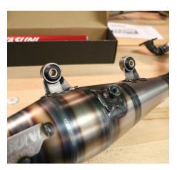
Install the exhaust bracket facing outside of the chamber. This is the only way the fixing holes matches the Minarelli Horizontal engine. The bracket should be hiding the chamber holders. **Do not tighten anything until the exhaust is correctly adjusted.**
